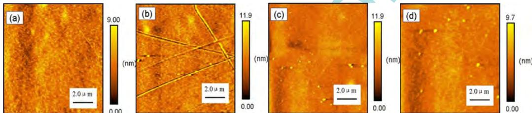
Fig. 1. AFM images of Ag films with different thicknesses on PET Sub.: (a)15nm, (b)30nm, (c) 75nm and (d)120nm.
