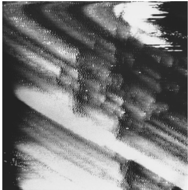
FIG. 3. The STM image of microcrystalline cellulose Sigma cell type 50. V_{\text{bias}}=475 mV, I_{\text{ref}}=0.81 nA. Scan area 40\text{ nm}\times 40\text{ nm} .
